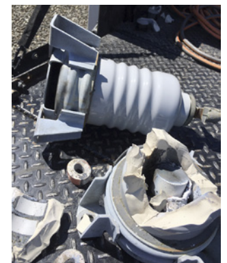
Lightning arrestors help protect from overvoltage events. These did their job at the Airport Substation after the car vs. pole accident on May 8.
